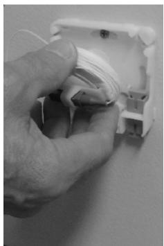
5. LOAD THE 25M FIBER SPOOL SO THAT THE (3) SPOOL LATCHES ENGAGE THE INNER SPOOL LIP AND SPINS FREELY.
